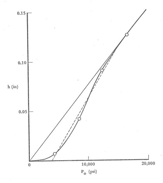
Figure 8. Variation of slot depth with jet pressure for Wilkeson sandstone at a feed rate v = 40 in/sec.
